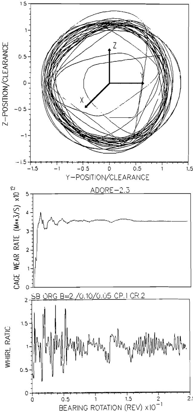
Fig. 3(b)—Bearing performance parameters with an outer race guided cage with a guide clearance of 0.20 mm and pocket clearance of 0.10 mm.
