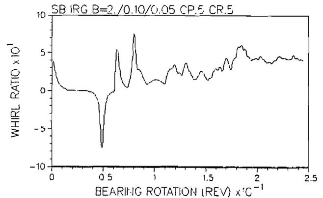
Fig. 6(a)—Bearing performance parameters with an outer race guided cage with a guide land and pocket clearances of 0.50 mm.
