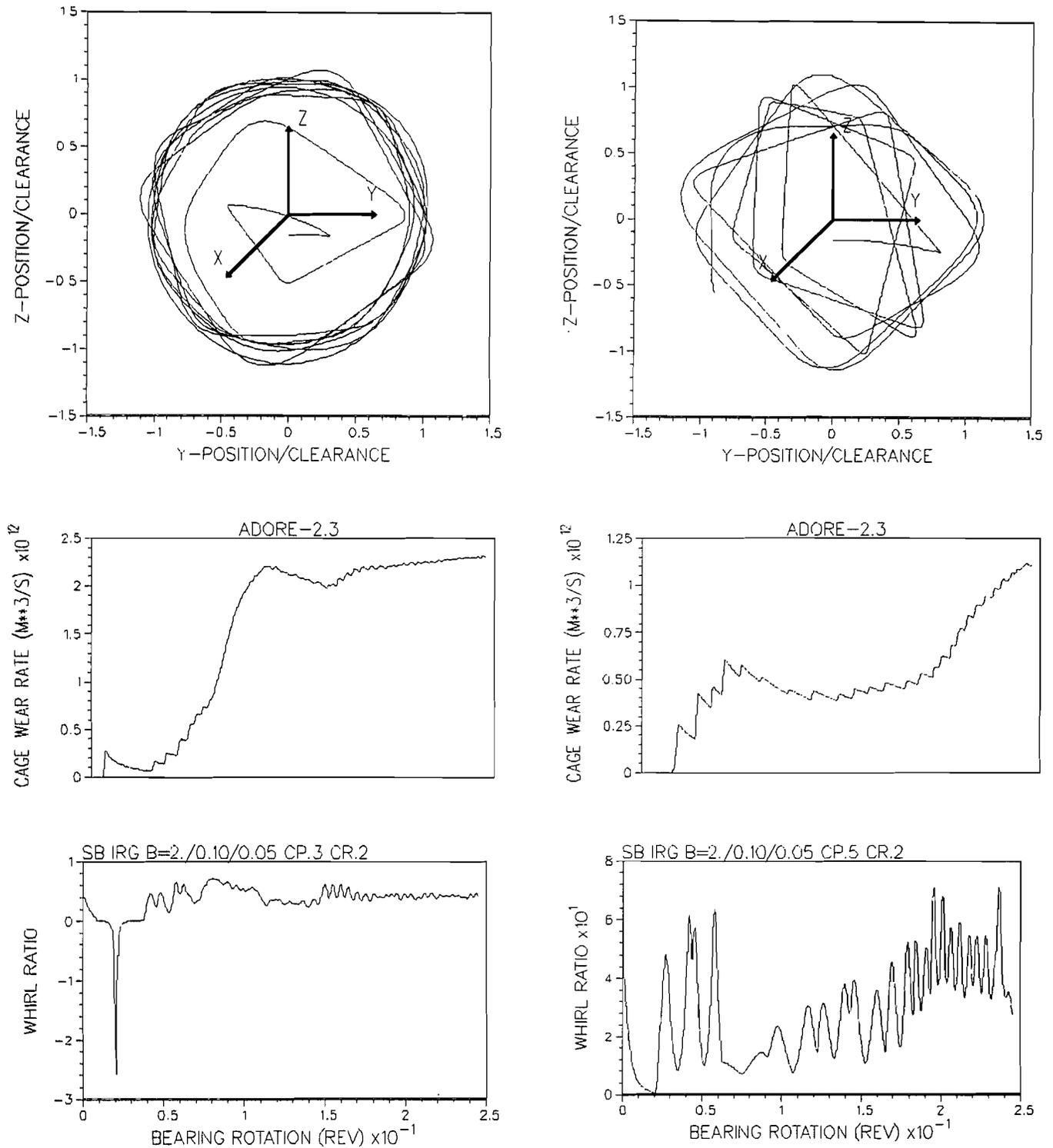
Fig. 5(a)—Bearing performance parameters with an inner race guided cage with a guide clearance of 0.20 mm and pocket clearance of 0.30 mm.
