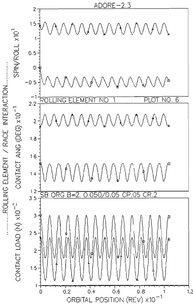
Fig. 2—Ball/race contact loads, angles and spin/roll ratios.
