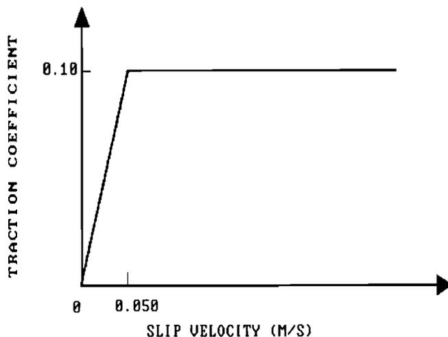
Fig. 1—Ball/race traction-slip relation.
