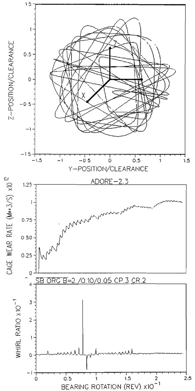
Fig. 3(c)—Bearing performance parameters with an outer race guided cage with a guide clearance of 0.20 mm and pocket clearance of 0.30 mm.
