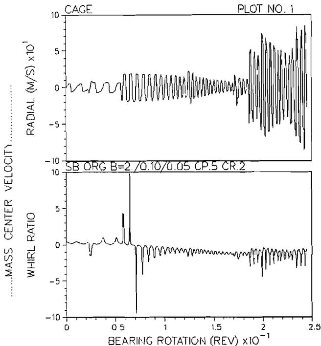
Fig. 4—Cage mass center whirl and radial velocities under unstable conditions.
