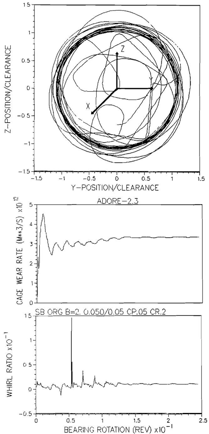
Fig. 3(a)—Bearing performance parameters with an outer race guided cage with a guide clearance of 0.20 mm and pocket clearance of 0.050 mm.
